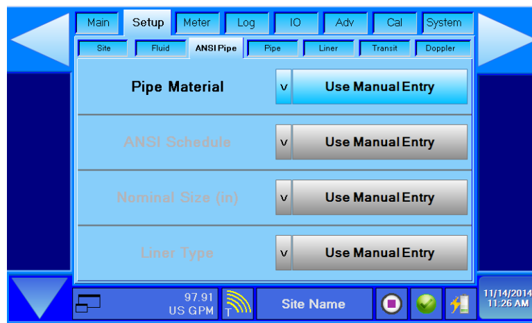
Figure 52: ANSI pipe page manual entry
