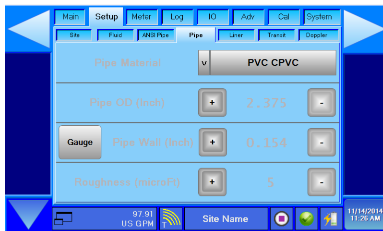
Figure 53: Pipe page from nominal entry
